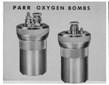
For more than fifty-five years, Parr oxygen bombs have been used in laboratories throughout the world for measuring calorific values and for determining sulfur and other elements in coal, oil, foods, rocket propellants and other combustible materials. New calorimeters and accessories are continually being added to extend bomb combustion methods into new fields and to improve the usefulness of this time-honored equipment. May we send you our latest Bomb and Calorimeter Catalog?
