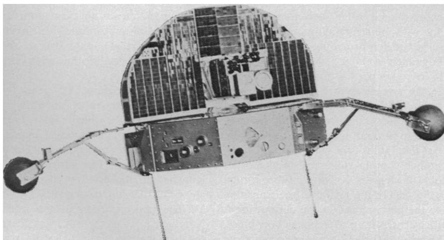
Fig. 3. The orbiting solar observatory OSO-IV; the diameter of the body of the satellite is about 4 feet (1.2 meters).
