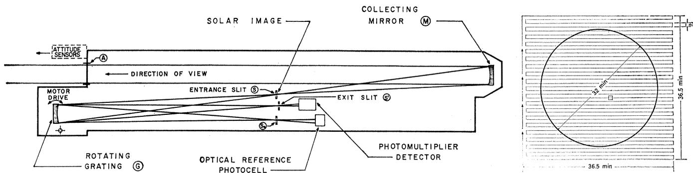
Fig. 4. (Left) Optical layout of the Harvard spectrometer aboard OSO-IV. (Right) Raster scanning pattern of the Harvard spectrometer over the solar disk. The small square represents the size of the square entrance aperture of the spectrometer.
