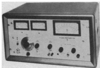
PHOTOMETER for photomultiplier operation with adjustable high voltage and sensitivities to the nano amp range.
