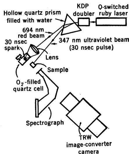
Fig. 1. Laser photolysis and spectroscopy in the nanosecond time range.
