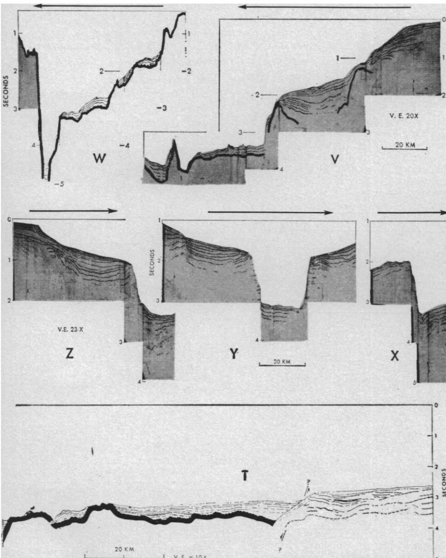
Fig. 3. Reflection profiles V, W, X, Y, and Z crossing fracture zones within the Gulf of California. Profile T crosses a transpeninsular fault under the Pacific west of the peninsula. Arrows match those of Fig. 4 and give positions and directions of the profiles; heavy black line, basement reflector.
