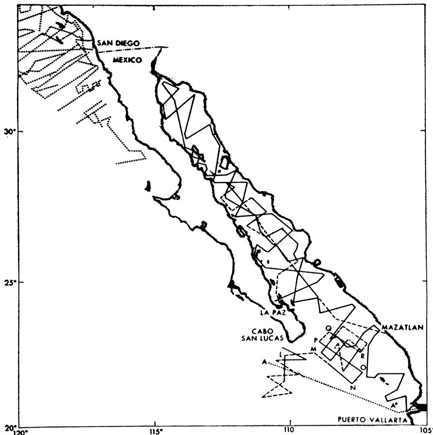
Fig. 1. Survey tracks in the Gulf of California and over the continental margin west of the peninsula. Both magnetic and reflection-profiling data were collected along tracks shown by solid lines; dashed lines show magnetic surveys only; dotted lines, reflection profiling only. Tracks off southern California are from earlier surveys. Positions of profiles in Fig. 2, A and B, are shown in the mouth of the gulf.
