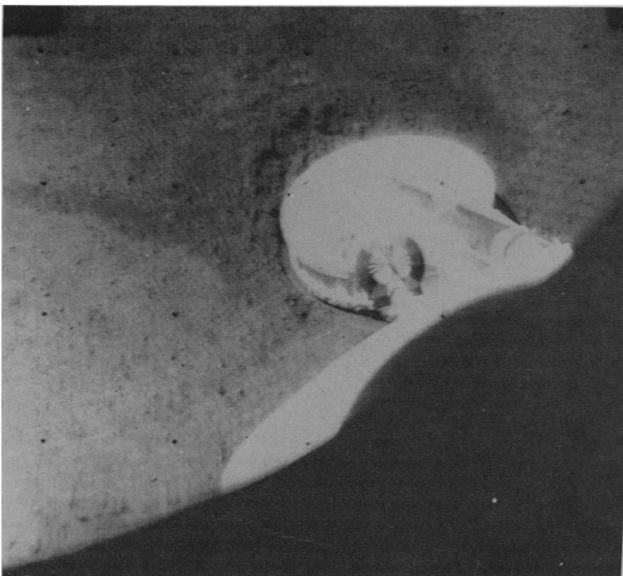
Fig. 1. Footpad of the Surveyor I spacecraft, showing the dark material thrown out by the impact of the foot on the lunar surface. [NASA photograph]
