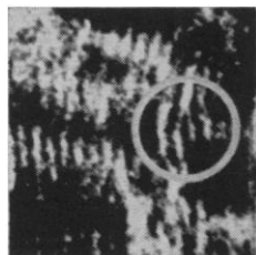
Layer planes of 3.4 AU spacing in graphitized carbon black. A dislocation is seen in the circled area. R. D. Heidenreich, Bell Laboratories.
