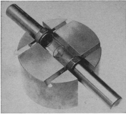
Fig. 1. Short-arm rotor with 100-ml polycarbonate centrifuge tubes in place.
