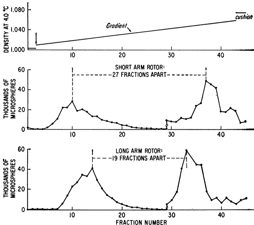
Fig. 2. With identical gradients and samples, the short-arm rotor improves separation between peaks, and resolution of the heterogeneous particles within peaks. The arrow indicates the sample-gradient interface. Centrifugation was carried out for 60 minutes with the long-arm rotor and 138 minutes with the short-arm rotor. The microscope count for fractions 29 to 45 is plotted  $\times 10$  to facilitate comparison of peak locations.
