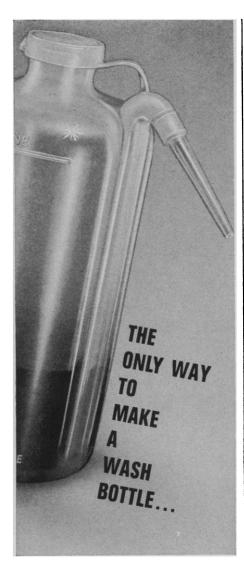
... with unitary construction—like the Nalgene® Unitary Wash Bottle. Dispensing tube and body are precision molded as a single unit—no seams, no leaks. And, it's easier to use—just squeeze to dispense to the very last drop. It's the only way to make a wash bottle—and we're the only people who make one this way. Nalge . . . innovator in plastic labware.
