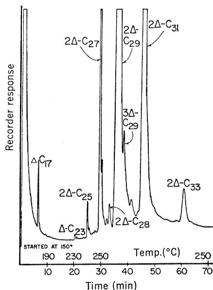
Fig. 1. Gas chromatographic separation of hydrocarbons of *Botryococcus braunii*, by use of an F & M 810 gas chromatograph equipped with a flame ionization detector. The glass column, 1.7 m by 0.3 cm inside diameter, was packed with OV-1 (methyl silicone fluid). The nitrogen pressure was 703 g/cm<sup>2</sup>; range was 10°; and attenuation was 2.
