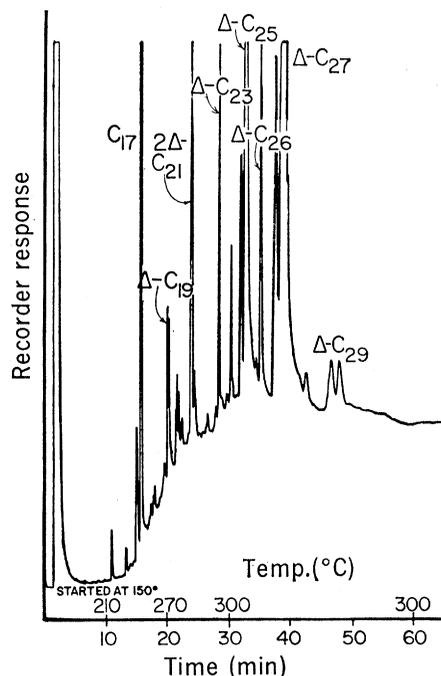
Fig. 2. Gas chromatographic separation of hydrocarbons of *Anacystis montana*, by use of an F & M 810 gas chromatograph equipped with a flame ionization detector. The capillary column was stainless steel tubing, 30 m by 0.025 cm inside diameter, coated with 10 percent Apiezon L (a high-temperature grease). The nitrogen pressure was 1406.0 g/cm<sup>2</sup>; range was 10<sup>3</sup>; attenuation was 1.
