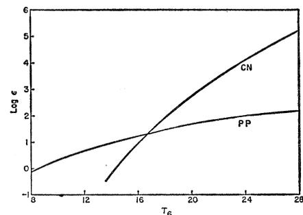
Fig. 4. The energy production, in erg/sec, as a function of the temperature in millions of degrees. For the proton-proton reaction (P P) and the carbon-nitrogen cycle (C N). Concentrations assumed  $X = Y = 0.5$ ,  $Z = 0.02$ . Calculated from Tables 8 and 9 of Reeves (12).
