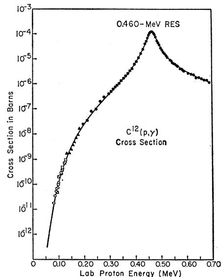
Fig. 3. Cross section for the reaction  $C^{12} + H$ , as a function of the proton energy. [From Fowler, Caughlin, Zimmerman (5)]
