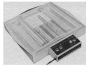
in polarity indicator and reversal switch, polarity indicator lights, full-length platinum electrodes, double-sloped transparent lid, and micro-switch safety attachment to lid for current cut-off. Special accessories are available for micro-immuno techniques. Size: 14" x 12" x 3½". In stock. Send for data sheet and complete catalog of TLC/TLE equipment to Shandon Scientific Company, Inc., 515 Broad Street, Sewickley, Pa. 15143 (Pittsburgh District).
