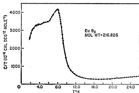
Fig. 1. Heat capacity of  $\text{EuB}_6$ .
