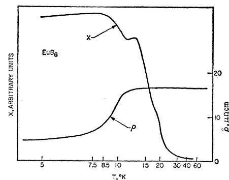
Fig. 2. Initial susceptibility ( $\chi$ ) and resistivity ( $\rho$ ) for  $\text{EuB}_6$ .
