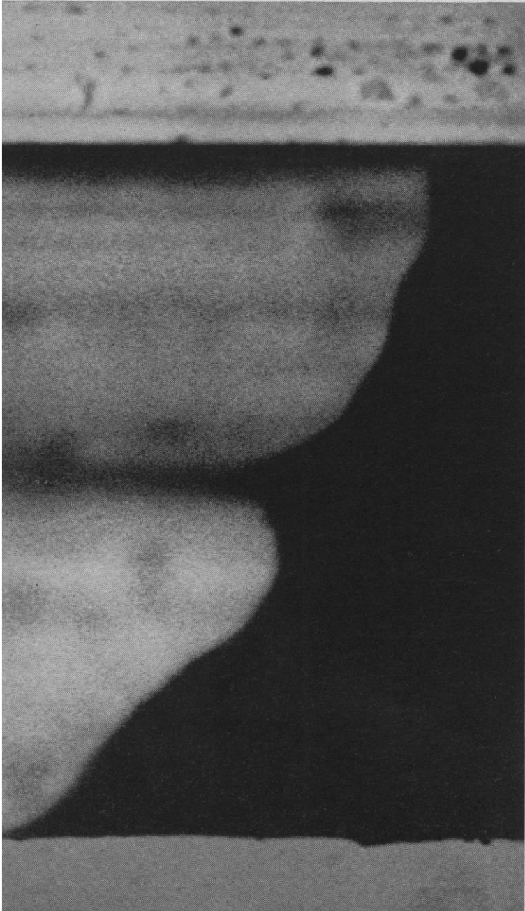
Illustration of an enlarged cross section of emulsion mask, 4 microns thick, showing ragged, sloping edge of opaque area. It is the slope of the emulsion edge that causes some fuzziness in transfer of the image to the silicon. Portion above large emulsion area is glass. The portion below is silicon.
