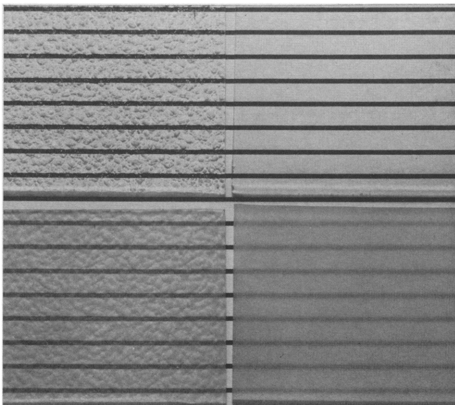
Fig. 2. Glass specimens used to demonstrate additivity of deformation and abrasive components of friction, photographed over a ruled background to accentuate the texture (see text).
