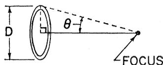
Fig. 3. Annular ring mirror (geometry B).
