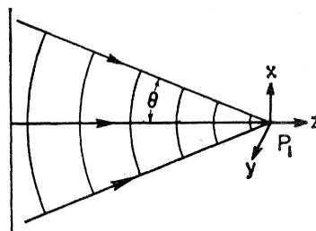
Fig. 1. Wave fronts converging on a focal point  $(x,y,z)$  from an optical system of angular aperture  $2\theta$ , where  $\theta$  is the polar angle of the array-circle;  $x$  is the displacement from the center of the diffraction pattern. The calculation is along one direction only.
