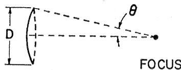
Fig. 4. Conventional parabolic disk (geometry C).
