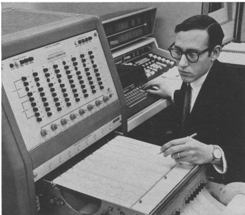
Scientist Barry J. Karafin of Bell Laboratories checks chart recorder waveforms from a BLODIB simulation. Karafin uses the computer console at his right to interact with the simulation program. This feature was developed for the BLODIB program to give users the flexibility of making changes in such things as component values without having to re-program an entire system.
