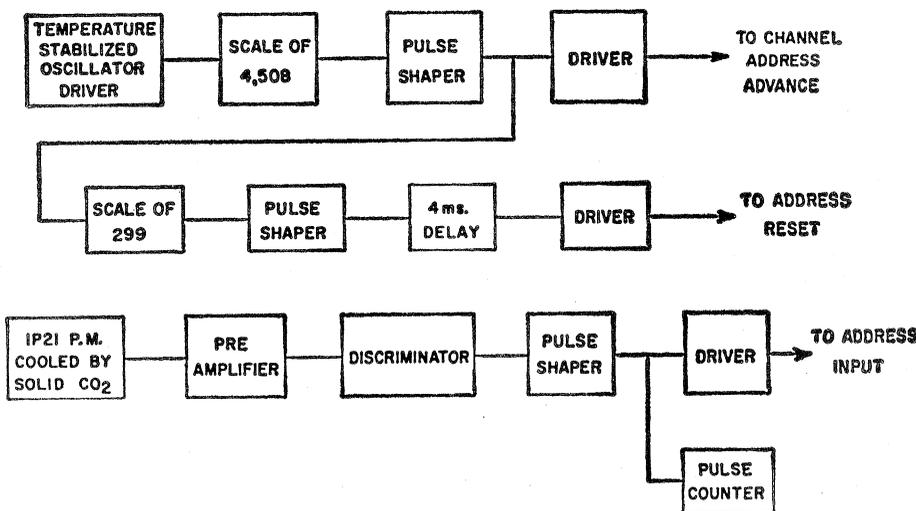
Fig. 1. Block diagram of the data-handling system. The master oscillator frequency was 1.008007 Mhz at the time of the experiment.
