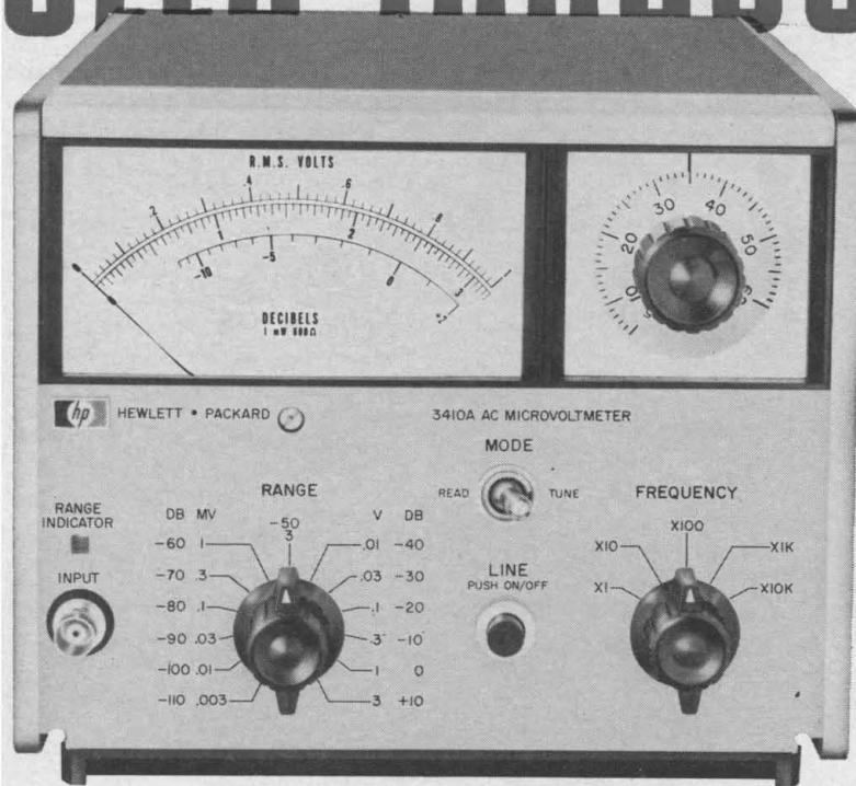
Measure 1 \mu V, 500 kHz signal out of 40 dB noise.
