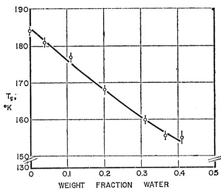
Fig. 1. Depression of the vitrification (glass-transition) temperature,  $T_g$ , of glycerol ( $184^\circ \pm 1^\circ\text{K}$ ) by addition of water. A smooth line has been drawn through the experimental points in order to reduce the error in the graphic procedure for the estimation of  $T_g$  for pure water.
