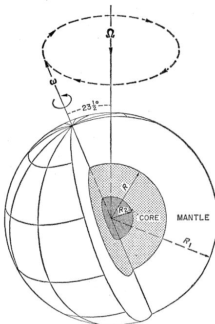
Fig. 1. The precessing earth. The angular rotation vector  $\omega$  is  $10^7$  times as large as the precession vector  $\Omega$ . The dynamic ellipticity of the core is three-fourths as large as that of the mantle.
