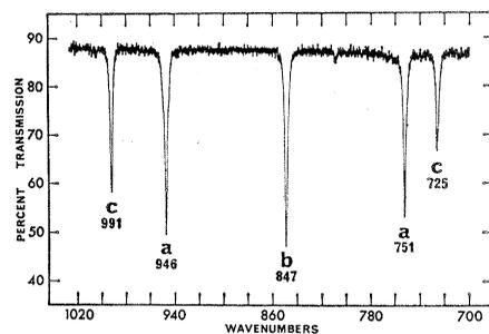
Fig. 1. Infrared PMI spectrum, 20°K, of a mixture of  $d_2$ -ethylenes at 1 percent in nitrogen (700 to 1025  $\text{cm}^{-1}$ ). (a) (1,1) Ethylene- $d_2$ ; (b) *cis*-(1,2) ethylene- $d_2$ ; (c) *trans*-(1,2) ethylene- $d_2$ . Twelve micromoles of ethylene mixture were deposited. Spectral slit, about 0.9  $\text{cm}^{-1}$ .
