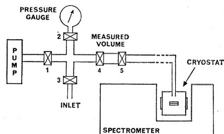
Fig. 2. Experimental configuration suitable for PMI studies. The volume defined by valves 4 and 5 should measure 15 to 16 ml. A glass line with stopcocks is suitable.
