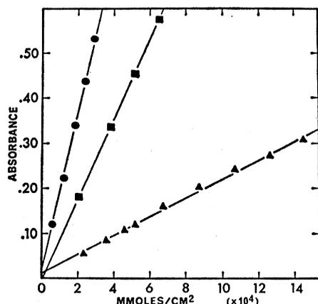
Fig. 3. A PMI Beer's law plot for the  $d_2$ -ethylenes. Symbols: ●, *cis*-(1,2) ethylene- $d_2$  (847  $\text{cm}^{-1}$ ); ■, (1,1) ethylene- $d_2$  (751  $\text{cm}^{-1}$ ); ▲, *trans*-(1,2) ethylene- $d_2$  (1295  $\text{cm}^{-1}$ ). The pulses of gas impinge on a substrate having an effective cross section of 19.5  $\text{cm}^2$ . The orifice through which the gas streams is an unworked length of Pyrex tubing, 5 mm in internal diameter.
