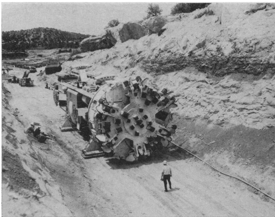
Fig. 3. Continuous, mechanized equipment to mine deeply buried ores economically in the future may resemble this 5-meter boring machine, linked to extendable conveyors to remove the broken ore.
