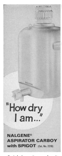
Can't leak, won't ooze, doesn't dribble-because the threaded boss is integrally molded as part of the one-piece body. This precision molding technique assures no leaks, ever! Two Teflon\* O-rings provide a positive seal for the needle-type 1/2" spigot. Molded of conventional polyethylene in 1, 2, 5,  $6^{1}/_{2}$  and 13 gallon sizes. Excellent for handling acids, collecting and dispensing distilled water and other liquids.
