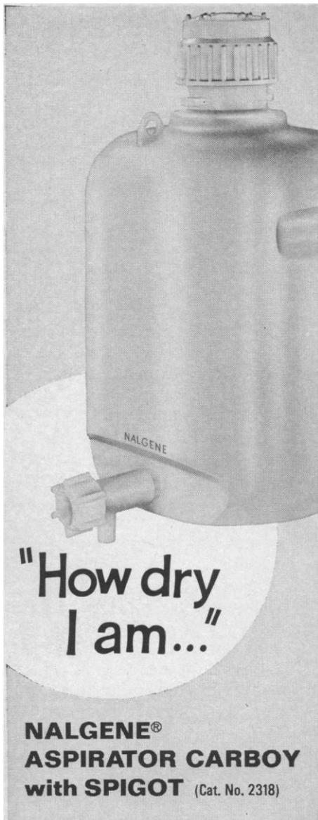
Can't leak, won't ooze, doesn't dribble—because the threaded boss is integrally molded as part of the one-piece body. This precision molding technique assures no leaks, ever! Two Teflon\* O-rings provide a positive seal for the needle-type 1/2" spigot. Molded of conventional polyethylene in 1, 2, 5, 6 1/2 and 13 gallon sizes. Excellent for handling acids, collecting and dispensing distilled water and other liquids.
