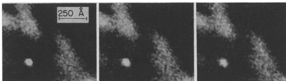
Fig. 3. Polytropic montage made by photographic superimposition of the component images in three different ways so as to accentuate the details lying at different levels in the specimen. With change in level, the gold-sol particle (bottom left) goes out of focus; virus particles, while maintaining a constant general arrangement, are changed with respect to their fine detail.
