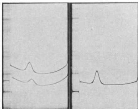
Fig. 1. Ultracentrifugal patterns of (left) the amorphous form (CPA) of *Chaetopterus* photoprotein at two different concentrations at 4.5°C and (right) the crystalline form (CPC) at 2.4°C. Speed, 59,780 rev/min; time, 64 minutes (CPC), 80 minutes (CPA).
