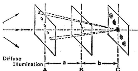
Fig. 1. Optical arrangement for obtaining autocorrelograms of an electron micrograph (A). B is a copy of A at  $b/(a+b)$  times the magnification, and oriented parallel to it. C is an unexposed photographic emulsion. The system is illuminated from the left with a diffuse source. All rays through corresponding points of A and B converge on the optical axis at C.
