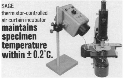
The Sage Air Curtain Incubator controls the temperature of specimens under the microscope within the range of  $30^\circ$  to  $40^\circ C$  with an accuracy of  $\pm$  0.2°C. It totally eliminates the need for enclosures of any kindmicroscope and specimen are completely accessible. Especially useful for biological studies of living materials.
