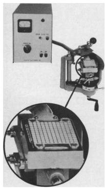
Thin, accurate tissue slicing by microtome with the "Tissu-Freez" attachment:
