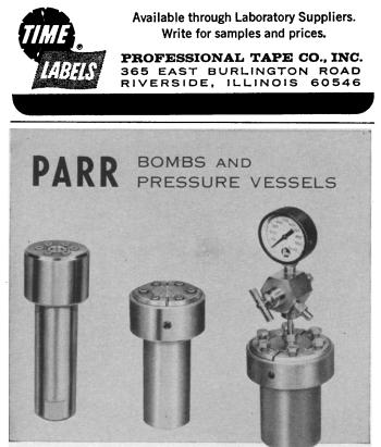
Parr offers a wide selection of bombs and pressure vessels for applying heat, pressure and agitation to any chemical reaction or physical test system. These are made in several different styles using a broad assortment of corrosion resistant alloys. Capacities range from 15 to 2000 ml. with working pressure limits of 1000, 3000, 7500 psig. and higher. Valves, thermowells, dip tubes and other attachments can be provided.
