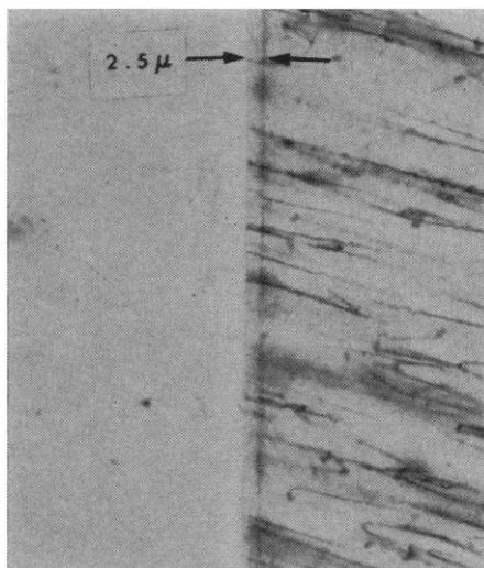
Fig. 1. Thin section of obsidian from Panum Dome, showing  $2.5\text{-}\mu$  hydration layer.
