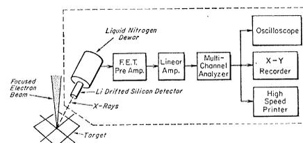
Fig. 1. Solid-state energy-dispersion spectrometer.
