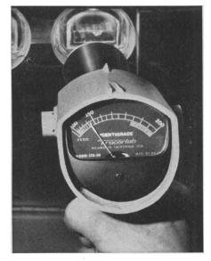
Pyrometer shows that Tracerlab's LTA-600 can ash samples thoroughly at temperatures well below 150°C — low enough to leave all inorganic constituents unaltered. A cold plasma of atomic oxygen does the ashing, while our accessory pyrometer keeps you posted on the temperature.
