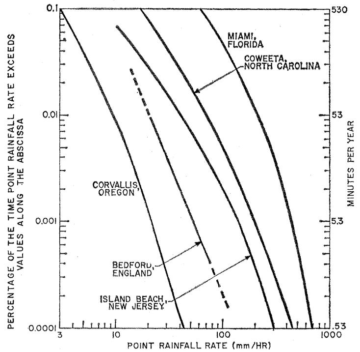
Fig. 4 (left). Rainfall rate at a point, as measured by a rain gauge with a time resolution of about 1 second. Fig. 5 (right). Yearly distributions, in percentage of time and in minutes per year, of point rainfall rates for various places in the United States and for Bedford, England. [Based on a 1-year data sample made available through the courtesy of the Illinois State Water Survey]
