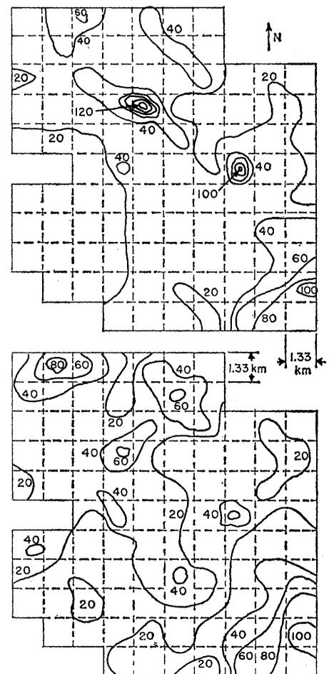
Fig. 9. (Top) Plot of rainfall-rate contours (in millimeters per hour) showing several rain cells on the Holmdel, New Jersey, rain-gauge network; (bottom) contours 10 seconds later.
