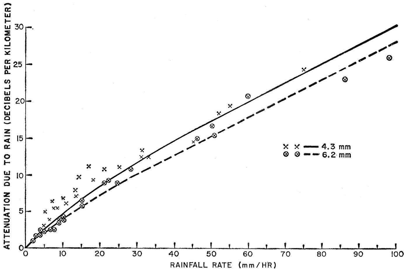
Fig. 3. Measurements (made by Bell Telephone Laboratories) of attenuation due to rain at wavelengths of 6.2 and 4.3 millimeters, compared with corresponding calculated values (solid and dashed lines).
