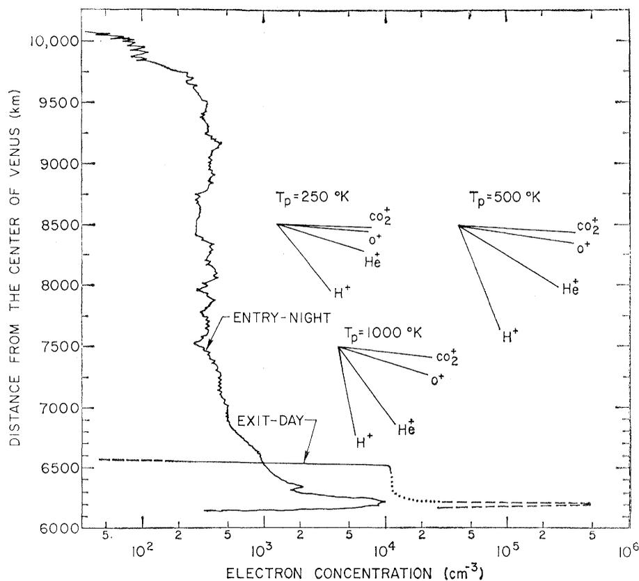
Fig. 3. Profiles of electron concentrations in the night and day ionospheres of Venus. The night profile and the solid part of the day profile are from integral inversion of the phase data. The dashed day peak is from very preliminary model-fitting to amplitude data. The dotted line is in an area where no direct measurements were made due to the formation of caustics.
