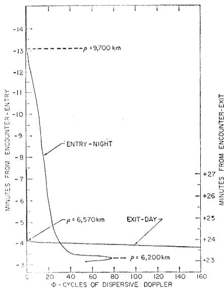
Fig. 2. Dispersive phase due to the ionosphere at entry and exit, plotted as a function of time and radius from the center of Venus.
