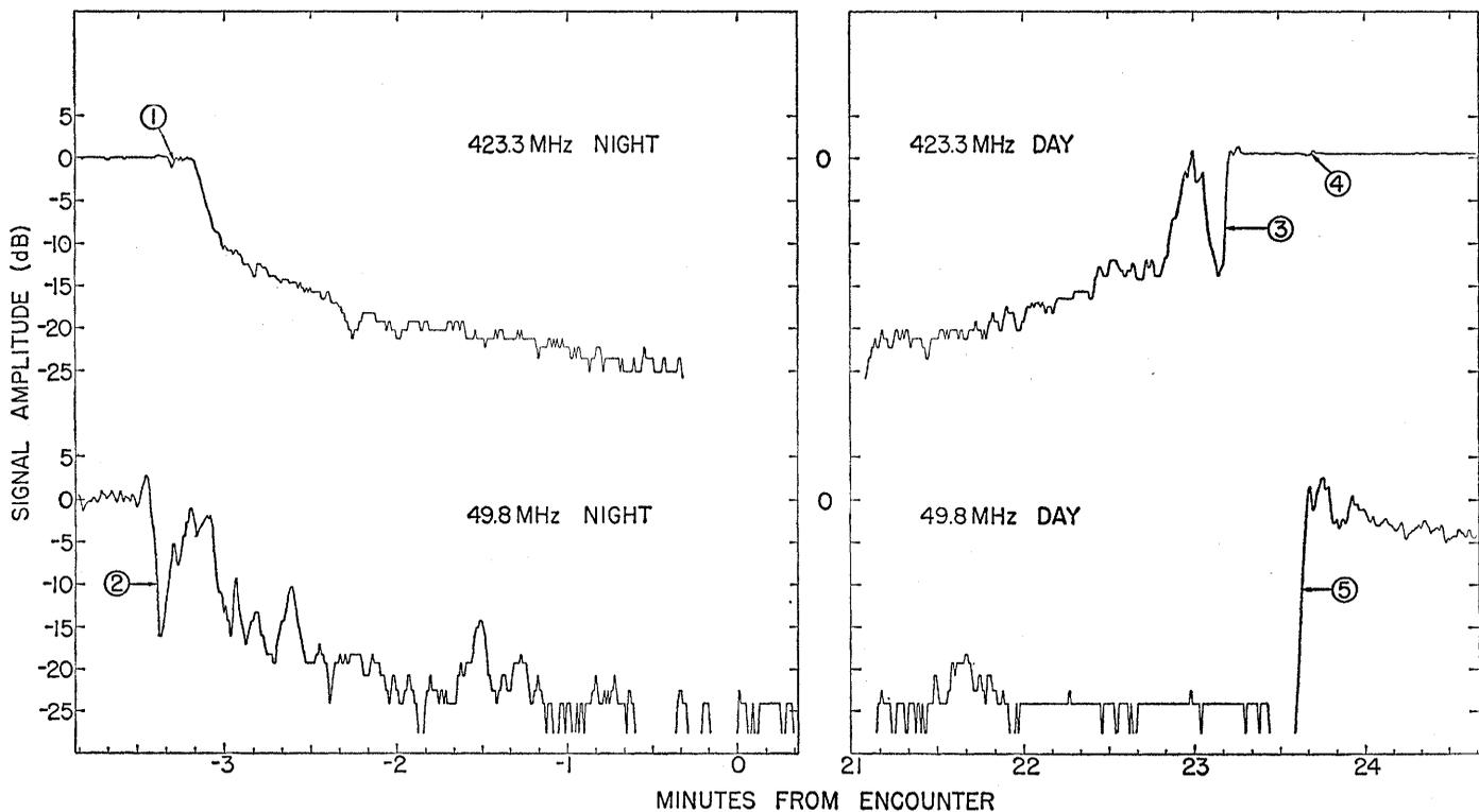
Fig. 1. Signal amplitudes at two frequencies during entry (nightside) and exit (dayside) occultation. Ionospheric effects are tagged 1 to 5, while the dense neutral atmosphere caused the general slow decay at entry and rise at exit.
