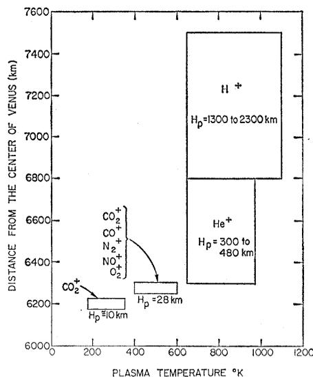
Fig. 4. Possible constituents and plasma temperatures for the nighttime upper atmosphere, derived from measured scale heights (upper three boxes) and preliminary model-fitting to the amplitude measurements (lower box).
