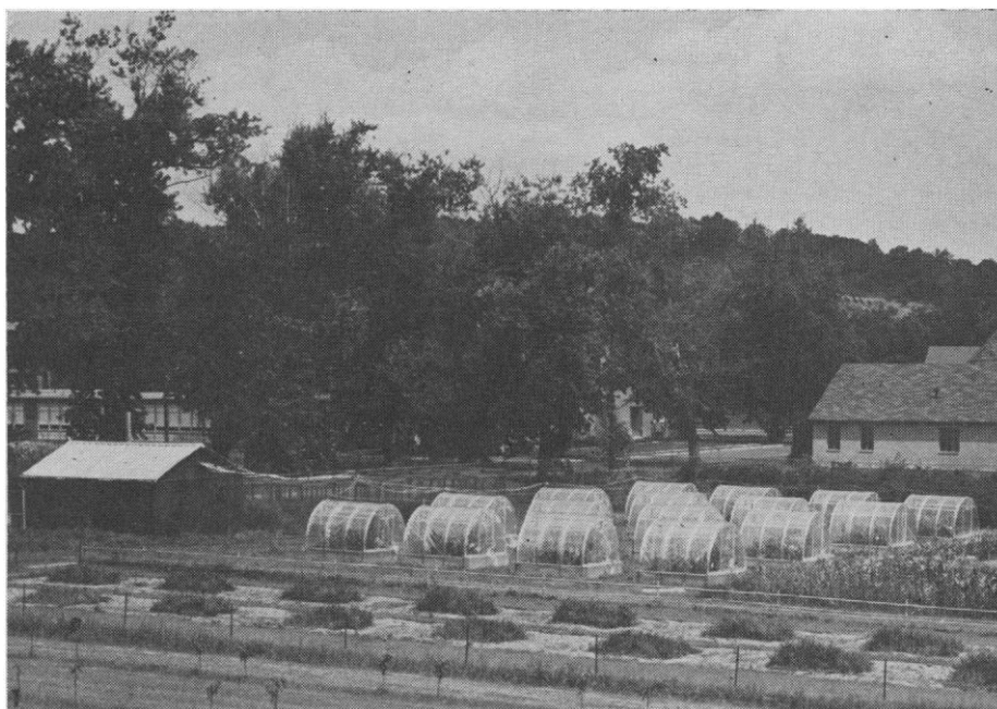
Field trial on the effects of air pollution by fluorides on photosynthesis and respiration of sorghum. Portable, plastic-covered houses are placed over the plants at the desired stage of growth and supplied with metered amounts of fluorine. The air in each house is automatically sampled for carbon dioxide content every hour through aluminum tubes running to the infrared analyzer in the shed.
