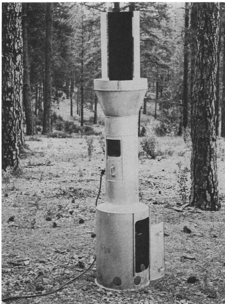
The response of free-flying bark beetles to pheromones (produced in logs, extracted from the beetles, or produced synthetically) is determined by olfactometers in the Institute's experimental forest at Grass Valley, California.
