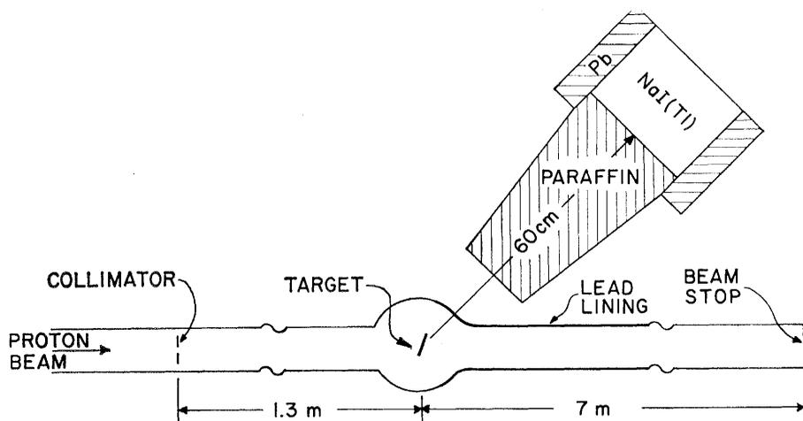
Fig. 1. Experimental arrangement for detecting the gamma rays from the radiative capture of protons accelerated by the tandem Van de Graaff accelerator at the Argonne National Laboratory.
