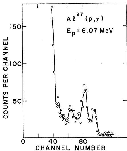
Fig. 2. Pulse-height spectrum observed in the NaI(Tl) crystal when an aluminum target with a thickness of 200 micrograms per square centimeter is bombarded with 6.07-Mev protons.
