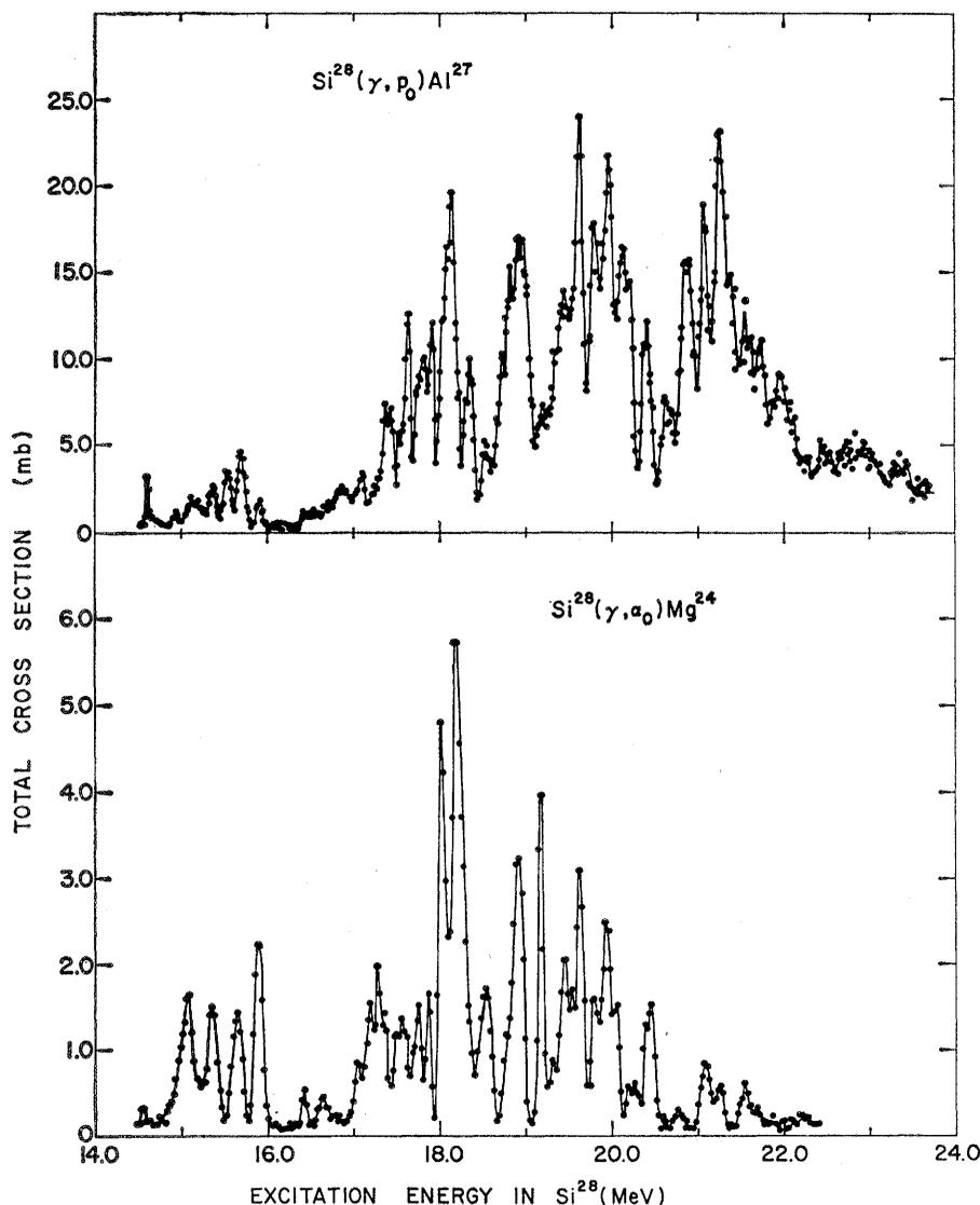
Fig. 8. Comparison of the  $Si^{28}(\gamma,\alpha)$  and  $(\gamma,p_0)$  cross sections. The data are from the radiative-capture experiments, but they have been converted to the inverse reactions by use of the principle of detailed balance.
