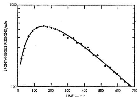
Fig. 1. Growth and decay of daughter Fm<sup>256</sup> fission radioactivity in an initially pure sample of Md<sup>256</sup>.
