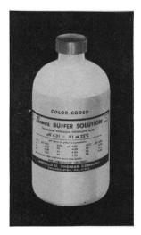
COLOR CODED BUFFER SOLUTIONS, Thomas. For precise pH meter calibration. A minute amount of colorant provides for immediate and certain visual identifica-tion, i.e., Red for pH 4, Yellow for pH 7, and Blue for pH 10.
