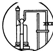
The Combititrator-3D can be set up to perform virtually any common or unusual titration: automatic potentiometric with recording; automatic potentiometric to an endpoint; constant-potential with recording of reagent volume against time (pH stat titration); pH and mV measurements; acid/base, redox, precipitation, non-aqueous, or complex titrations.
