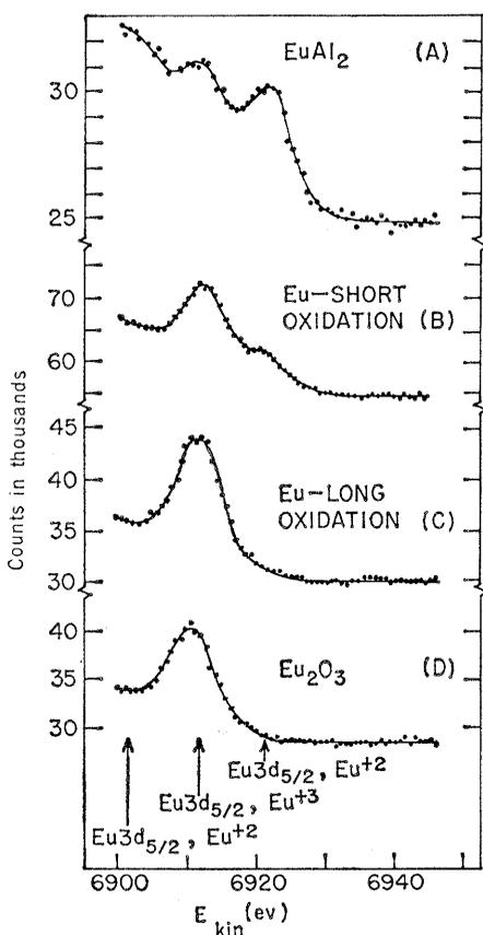
Fig. 2. Photoelectron peaks from various europium compounds. The two peaks for the 2+ state are due to excitation by two different x-ray lines. See text for details. The counts indicated on the ordinate were accumulated by counting for a total of from 2 to 4 minutes at each energy value.
