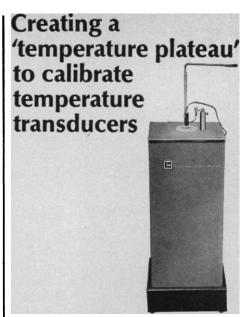
The L&N 8411 Fixed Temperature Standard consists of a vertical electric furnace and a cell containing a pure metal sample. It's virtually infallible in providing a known, fixed-reference temperature (such as the zinc-point) for calibrating resistance thermometers or thermocouples. Here's why.
