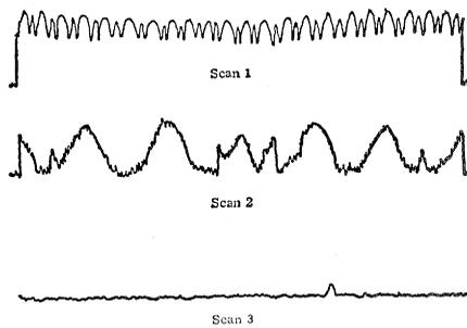
Fig. 3. Spectral scans illustrating the effect of optical baffling. Scan 1 is from a flight from Eglin Air Force Base, Florida, 29 January 1962; scan 2, from Fort Churchill, Canada, 18 July 1964; and scan 3, from White Sands, New Mexico, 13 November 1963. All scans are at heights greater than 100 km to eliminate the effects of rayleigh scattering.
