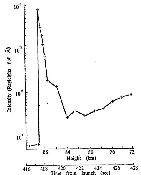
Fig. 2. Scattered light intensity as a function of time following detonation of an explosive charge to produce engine-payload separation.
