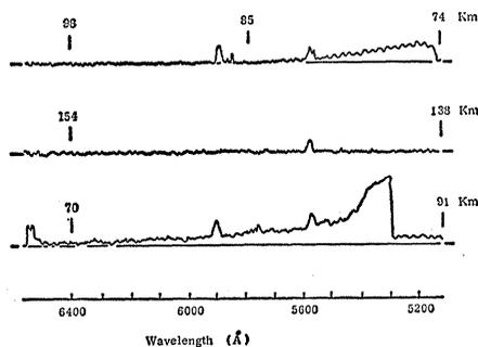
Fig. 1. Unreduced spectral scans from a rocket flight on 13 November 1963, White Sands, New Mexico. Heights at selected points on the scan are indicated above each scan. The top two scans are from the ascent portion, the bottom scan from the descent portion of the flight.
