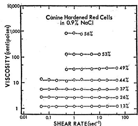
Fig. 1. A log-log plot of the relationship between viscosity and shear rate for suspensions of hardened canine RBC's in 0.9 percent NaCl. The cell percentages for the suspensions are shown for each curve. The viscosity values are essentially independent of the shear rate.
