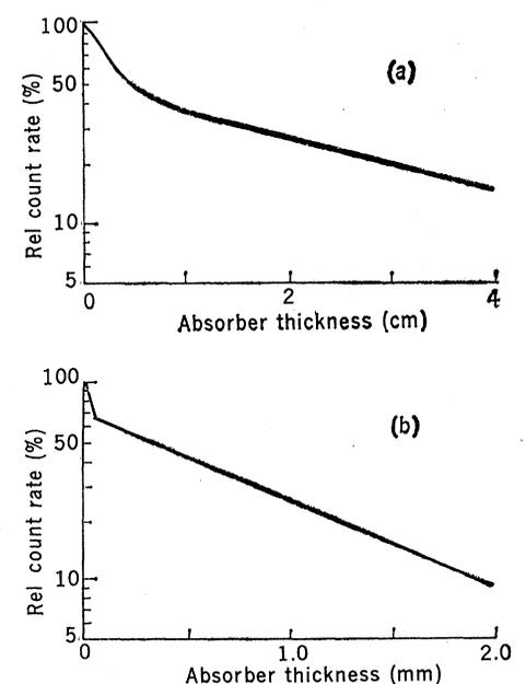
Fig. 2. Reduction in count rate as a function of added absorber thickness; (a)  $^{14}\text{C}$  bremsstrahlung; (b)  $^3\text{H}$  bremsstrahlung.
