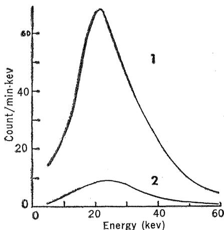
Fig. 3. Selected  $^{14}\text{C}$  bremsstrahlung spectra from rats. Curve 1, 100- $\mu\text{c}$  source in colon with the detector over the ventral surface. Curve 2, 100- $\mu\text{c}$  source diffused throughout body; detector over ventral surface.
