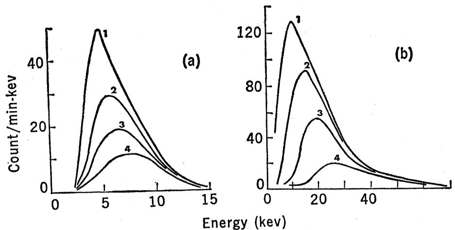
Fig. 1. Bremsstrahlung spectra as a function of added absorber thickness. (a)  $^3\text{H}$ ; (b)  $^{14}\text{C}$ . The numbers on the spectra refer to values of  $E$  marked with superscripts in Table 1.
