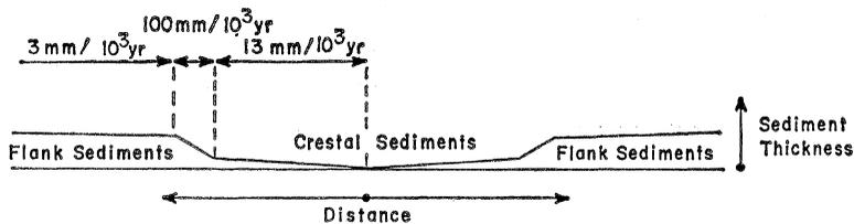
Fig. 4. Generalized sketch of crestal and flank sediment thickness based on data from the equatorial Pacific. The slopes give accumulation rates as indicated if spreading is assumed constant at 4.5 cm/yr.
