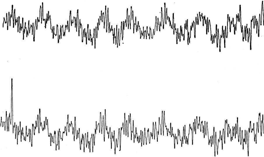
Fig. 1. (Top) An interferometer pattern from the source 3C-294 obtained directly while a recording was being made. (Bottom) An interferometer pattern from the source 3C-294 obtained on playback. The recorded signals were those correlated directly to produce the pattern in the top part of the figure.
