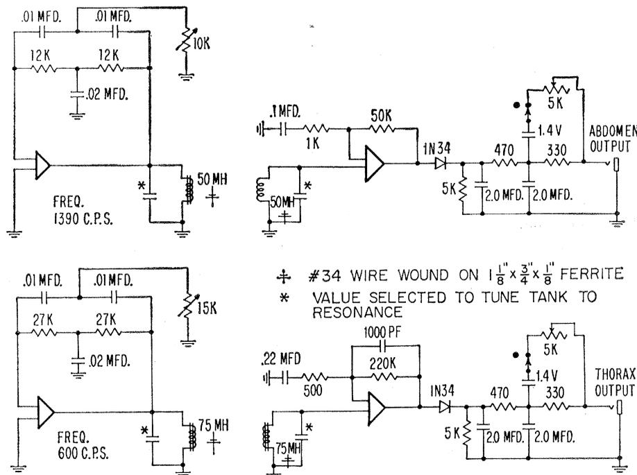
Fig. 1. Wiring diagram and coil specifications for the transducers.
