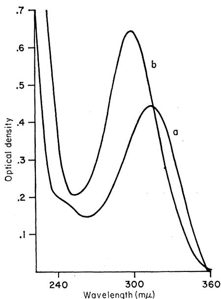
Fig. 2. The ultraviolet absorption spectra of  $P_2B$  (a) in neutral and  $pH$  2 solutions and (b) in  $pH$  12 aqueous solution.
