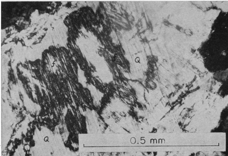
Fig. 6. Quartz, with embayed feldspar, from a granitic gneiss from Ries Crater (Bollstadt quarry), showing two sets of closely spaced fractures cutting across the quartz and the plagioclase but terminating at the boundary of the quartz grain.
