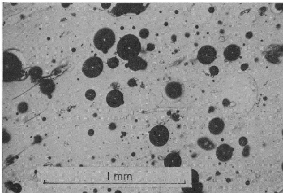
Fig. 4. A brown, transparent glass showing well developed schlieren and inclusions of serpent-shaped lechatelierite. There is no undissolved magnetite, and magnetic intensity of the glass is zero; black spherules are bubbles in the glass. Otting quarry, Ries Crater; plain polarized light.
