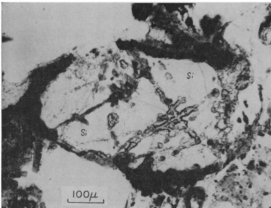
Fig. 3. A grain of silica glass (Si), with stringers of coesite (c), from a shocked, vesicular, biotite-granite gneiss. The silica glass is surrounded by a fused, opaque area of iron oxide.
