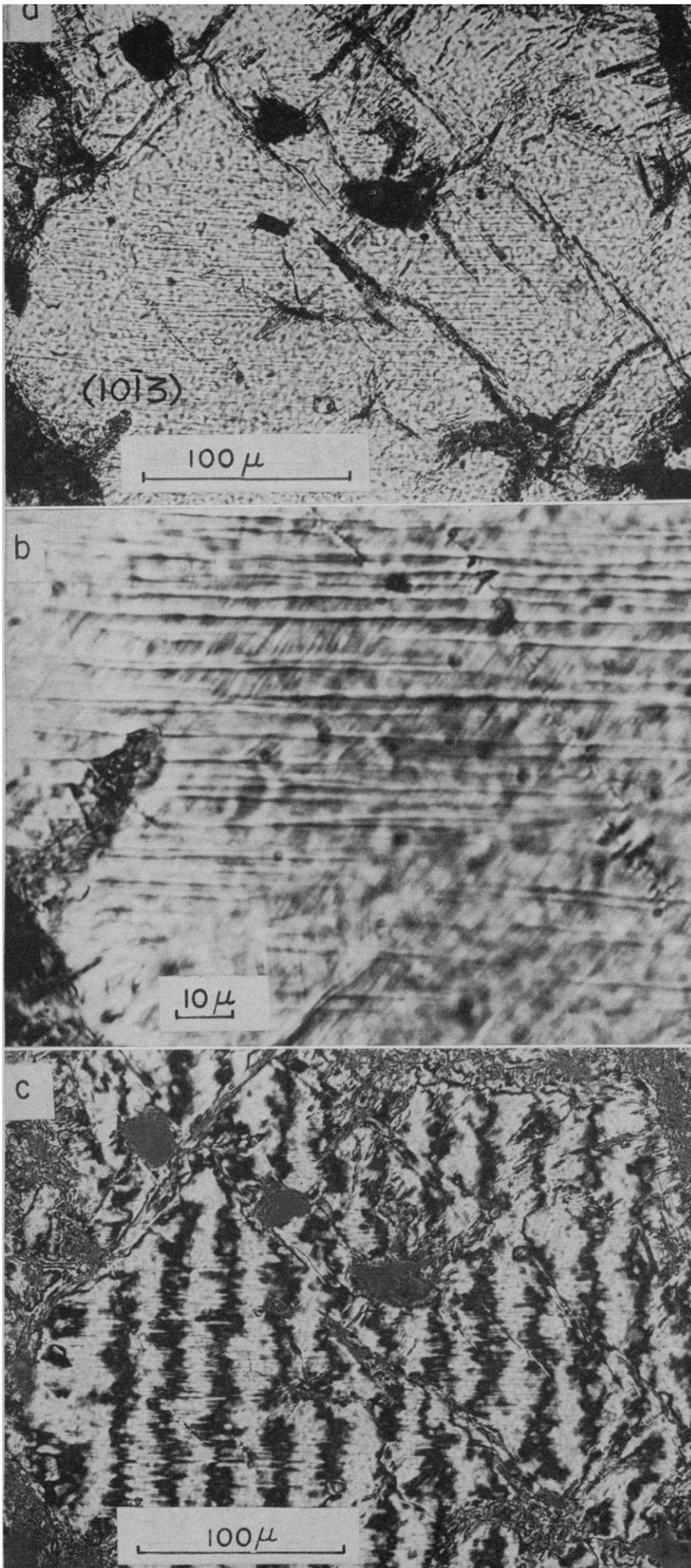
fer in that the glassy bands in shocked quartz are broader, and the difference in birefringence across them is greater. Furthermore, the mean index of refraction of a shocked quartz may be much lower than the mean index of refraction of quartz, than that of the statically deformed quartz of Christie *et al.*
