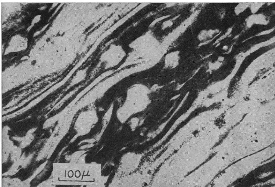
Fig. 8. A dark-gray, banded, magnetic glass in suevite from Ries Crater (Otting quarry). The dark bands contain many small particles of magnetite. Plain polarized light.
