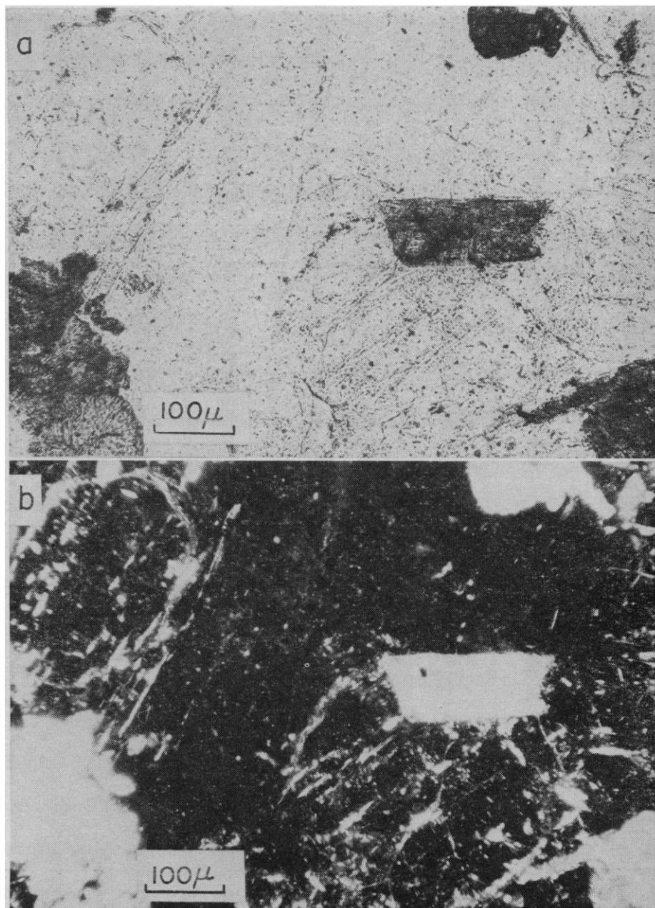
Fig. 7. (a) Plagioclase amphibolite showing the euhedral thetomorphic plagioclase glass in an anhedronal feldspar glass; the amphiboles remain crystalline. Plain polarized light. (b) Same field as (a); crossed nicols. The euhedral thetomorphic plagioclase is revealed by the birefringent micaceous mineral along the crystal boundary and cleavages.
