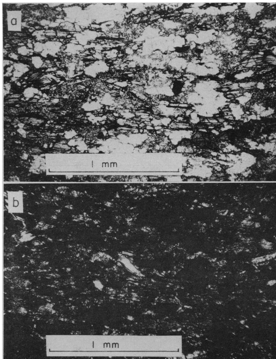
Fig. 2. (a) A shocked biotite-quartz schist. The quartz has been selectively transformed to theomorphous silica glass (white areas); the biotite remains crystalline. Transmitted polarized light. (b) Same field as (a); crossed nicols. The silica glass is isotropic and biotite remains birefringent.
