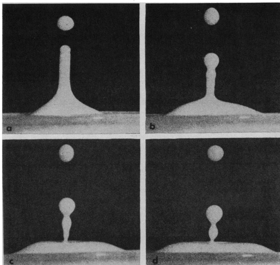
Fig. 2. The amplification of an unstable wave on the surface of a liquid jet. The time intervals between the photographs are 0.01, 0.006, and 0.005 second, respectively ( $\times 2.5$ ).
