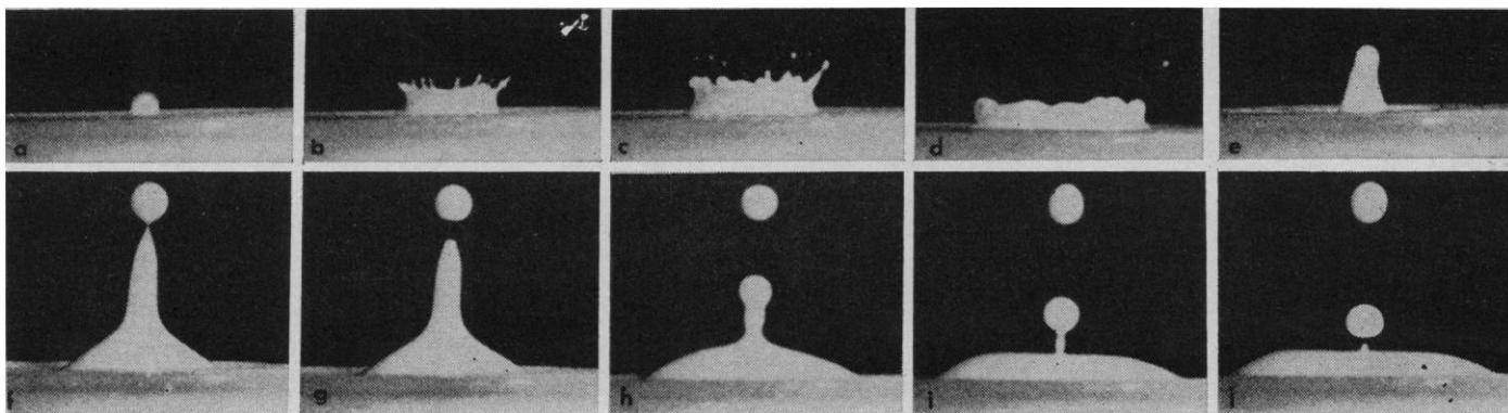
Fig. 1. The sequence of events following the impact of a drop approximately 3.4 mm in diameter on a plane surface of liquid ( $\times 2.5$ ).
